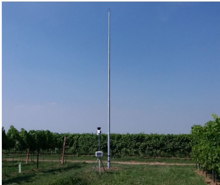
Fig. 10b Completed installation, weather station equipped with sensors for temperature, humidity, precipitation, wind direction and intensity, leaf wetness, soil temperature and humidity.
